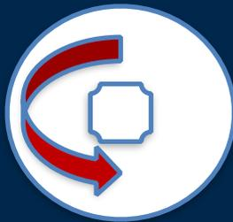
Handle turns Counter-clockwise to increase temperature
